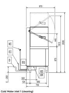
D Drain Electrical inlet (power) EO Electrical Outlet HWI Hot water inlet Water inlet WI
